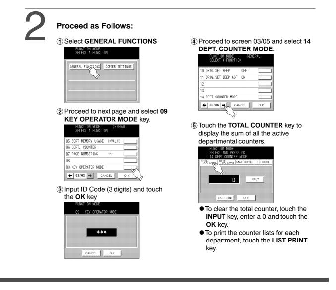
• To reset the function mode, press the **RESET** key.
