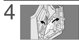
Automatic Duplex Unit (ADU) ① Open the Paper Feed Guide. ② Remove the misfed paper.
