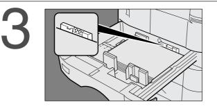
Make sure paper is not loaded above the overfill indicator located in the Paper Tray.
