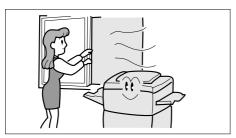
■ The copier should be installed in a well-ventilated area to minimize the ozone density in the air.
