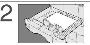
Place the paper with the copying surface facing upward. Special papers, like glossy paper, mailing labels and transparencies cannot be used in the Paper Tray. Use the sheet bypass for special paper.
